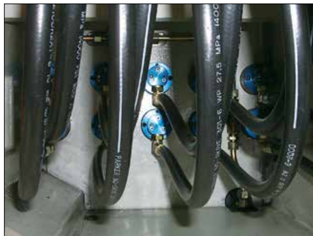
DEUBLIN 1117 Bearingless Unions on Automotive Transfer Line
