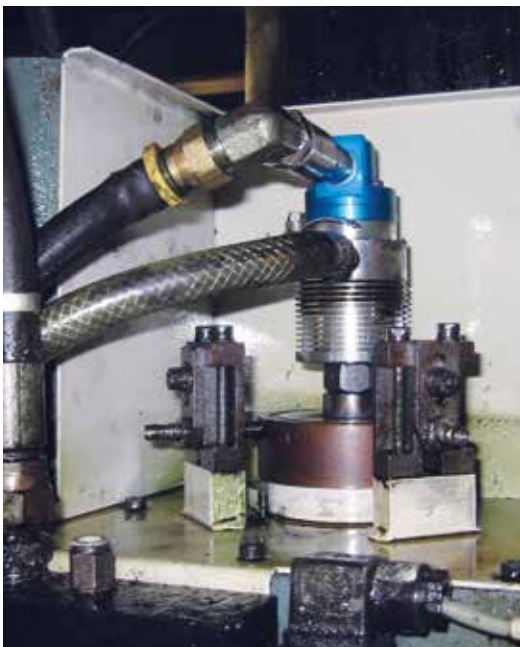
DEUBLIN 1109 on vertical machining center
