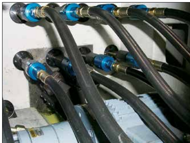
DEUBLIN 1116 Bearing-Supported Unions on Automotive Transfer Line
