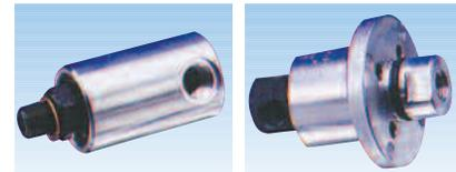
**Model 1115-000-001.** 11/32" capacity, maximum pressure 150 psi, max temperature 250°F, maximum speed 3,500 RPM. This model union is most commonly used when converting a vehicle to the CTIS system. The male thread can be attached to the solid axle and the supply air from the body to the tire. Shaft mounted conversions of this design are available, and illustrated on Page 34.
