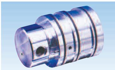
**Model 882, 2-passage union.** 1/8" pilot capacity and 5/16" supply air capacity. Operating data: Maximum air pressure 150 psi, max temperature 250°F, max speed 450 RPM. This 2-passage model was designed to be used where a wheel valve is required. The O-Ringed union body can be installed in the solid axle and air lines connected to the rotor head.
