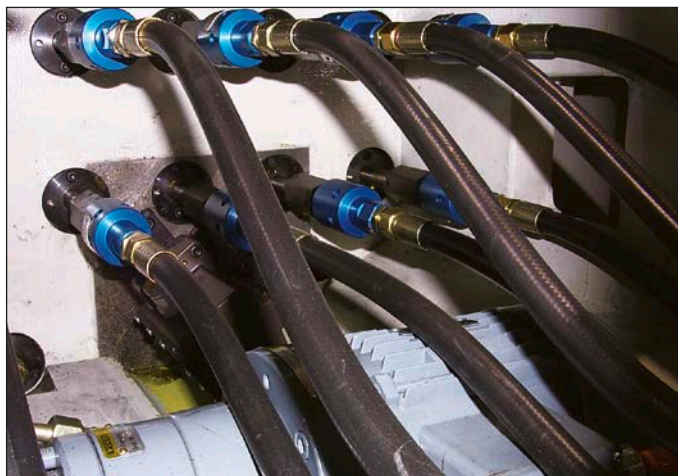
Deublin 1116 Bearing-Supported Unions on Automotive Transfer Line.
