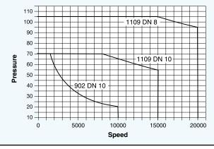
The curves in the adjacent diagram limit pressure and speed in relationship to one another. Within the given area the reliability of the rotating union is guaranteed provided that conditions specified elsewhere are upheld.
