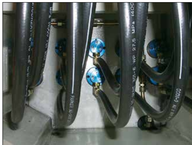
DEUBLIN 1117 Bearingless Unions on Automotive Transfer Line
