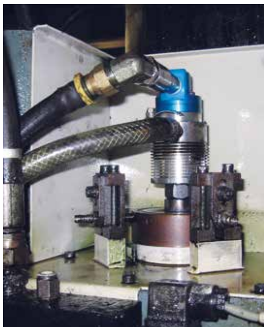
DEUBLIN 1109 on vertical machining center
