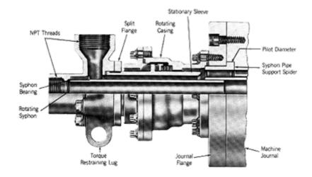
The Series 300 Rotary Joint has the following special features:
