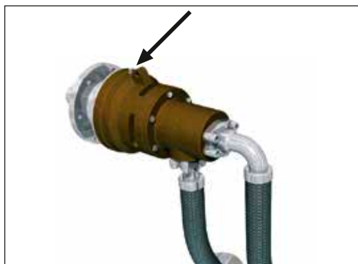
Fig. 8: Attach grease gun for relubrication
