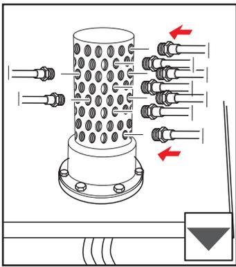
Attach appropriate, flexible hose with sealant or PTFE tape. No rigid piping as it may create excessive side loads and damage the union.
