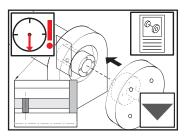
When mounting water supply cover with installed union make sure that the pin fits into the keyway of the rotor. Cover must be mounted flush.
