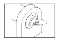
Ensure roll bore is clean and free of debris and burs.
