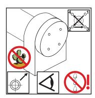
Check the union for leakage.
