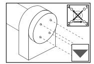
Secure the roll cover by tightening the screws in a star pattern.
