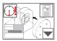
When mounting water supply cover with installed union make sure that the driving pin fits to the driving plane of the rotor. Cover must be mounted flush.
