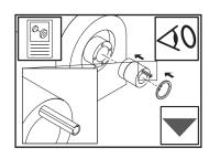
Insert bushing into the roll with axial driving pin outside. Secure with snap-ring (if supplied). Use technical drawing.
