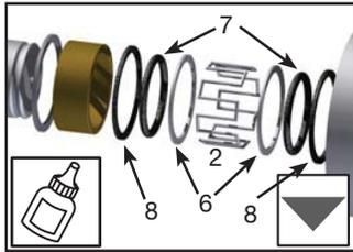
Apply silicone-based grease to all o-rings (7). Install backup washers (8), O-rings (7), seal guide (6), and to serpentine spring (2) housing (1).
