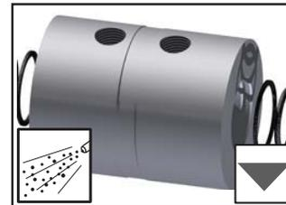
The housing (1) may be grit-blasted with glass bead or aluminum oxide to remove dirt and debris. **Sand-blasting is NOT recommended.**
