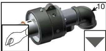
Plug and seal the rotor. Connect air hose to elbow port (10) and pressurize with 7 bar (100 psi) air.
