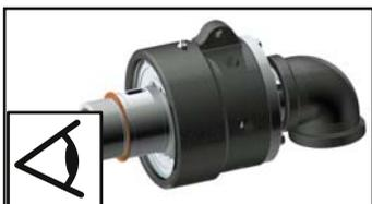
Apply soap to the Ø 3 mm diameter hole into the tape. Rotate union a few turns by hand. If no bubble rises up, then the union has passed the leakage test.
